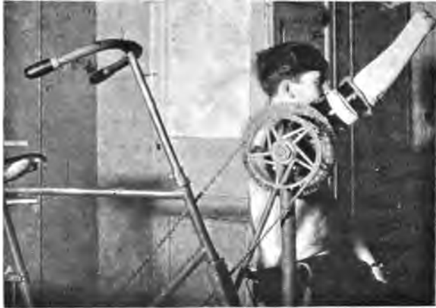
FIG. 79.—Measuring the power of a Stump (Arm) by means of the Dynamometrical splint.
